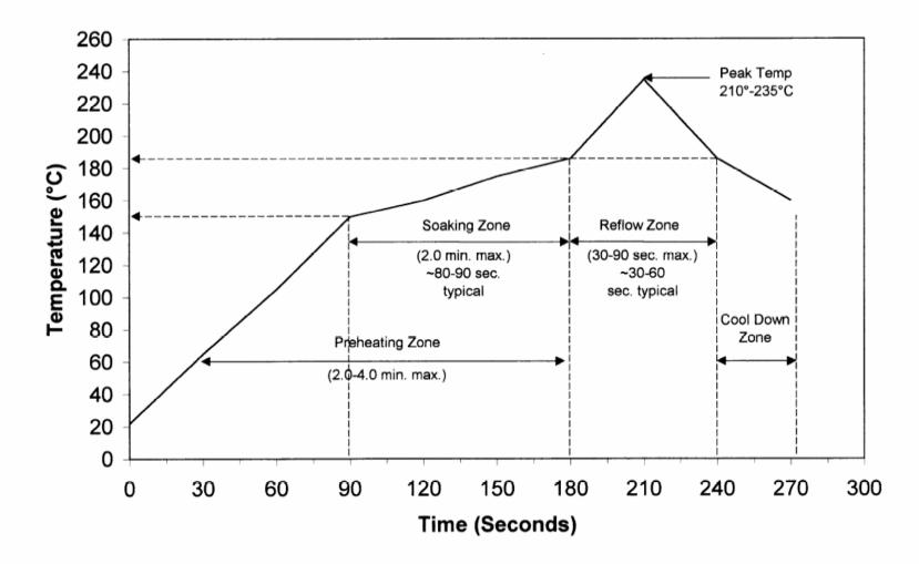
A typical reflow profile. In the first zone, preheating should not exceed 2.5C/sec to prevent solder ball formation or other defects.
